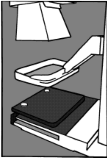
Fig. 2.3 Alignment of X-ray field/image receptor measurement
